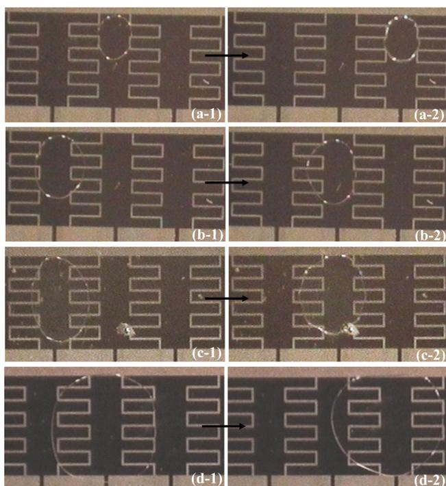
FIG. 4. Different volumes of droplets transported from left to right under same driving signal in a parallel-plate EWOD device with rectangular interdigitated fingers: (a) 27 nl, (b) 57 nl, (c) 90 nl, and (d) 190 nl.
