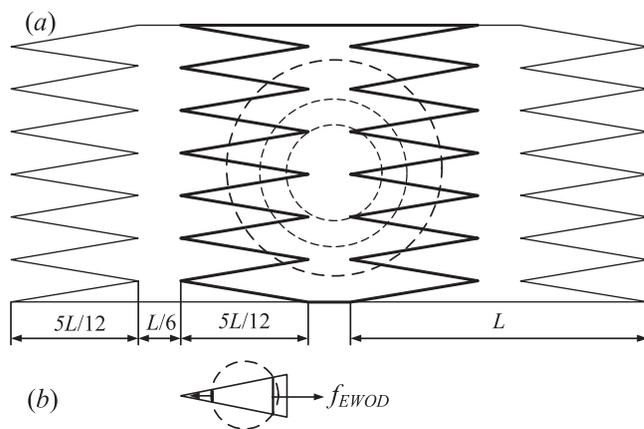
FIG. 6. (a) EWOD electrode with triangle fingers for size-variable droplet actuation, (b) the mechanics demonstration of small droplet actuated by large triangle fingers.
