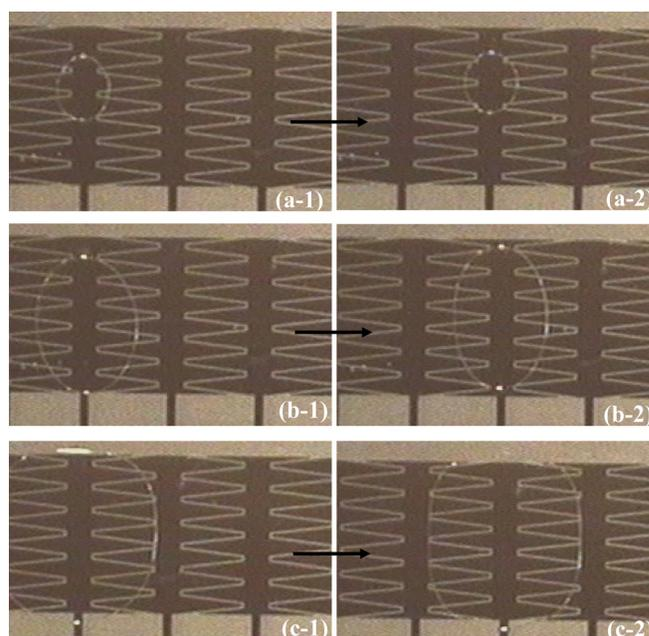
FIG. 7. Different volumes of droplets transported from left to right under same driving signal in a parallel-plate electrowetting device with triangle interdigitated fingers: (a) 15 nl, (b) 90 nl, and (c) 180 nl.<sup>21</sup>
