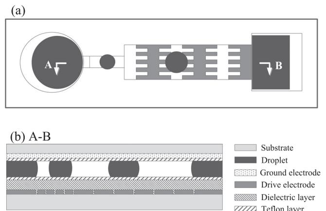
FIG. 3. Schematics of parallel plate EWOD device configuration with the EWOD electrode proposed.
