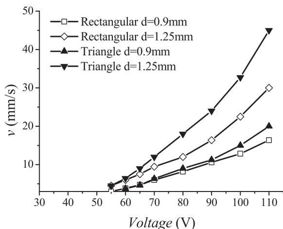
FIG. 8. Voltage-dependent velocity indicating faster transporting of electrode with triangle fingers than that with rectangular fingers for droplets in relatively large size.
