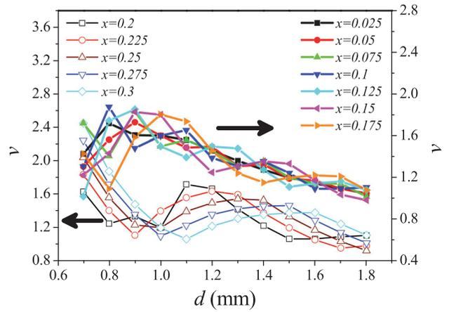
FIG. 2. Theoretical calculation of droplets velocity affected by finger width and droplet diameter.
