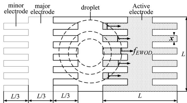
FIG. 1. EWOD electrode with rectangular fingers for size-variable droplet actuation.
