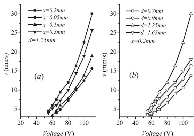
FIG. 5. Driving velocity affected by (a) rectangular fingers width and (b) diameter of droplets under different drive voltages.
