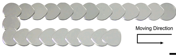
Fig. 4. Experimental observation of long-distance directional droplet motions. The stacked photo demonstrates the droplet movement with a 300 ms interval. See Movie. S3 in Supplementary Information for the original video. Scale bar: 1 mm.
